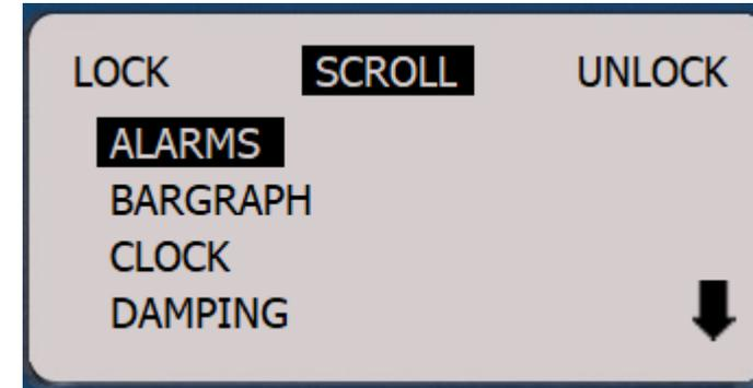
SCROLL using the up or down ARROW keys to highlight the options. Use the right or left ARROW keys to LOCK or UNLOCK. The end user will enter password to UNLOCK.
