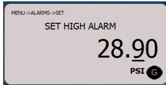
Once the alarm setpoint has been reached the high or low alarm icon will show on the display and background color will change to red to indicate an alarm status.
