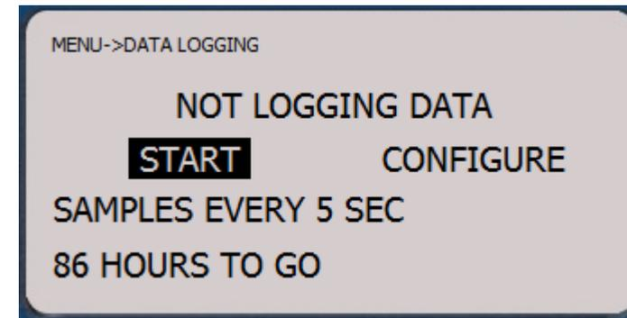
To change settings select CONFIGURE. The sample rate can be set from 1 second to 24 hours. Just use the arrows key to desired value and press SELECT to confirm.
