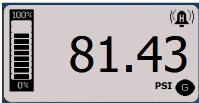
If you prefer not to use the bar graph, it can be turned OFF by using the RIGHT arrow key and pressing SELECT. *The bargraph will not be displayed with units measuring temperature.*
