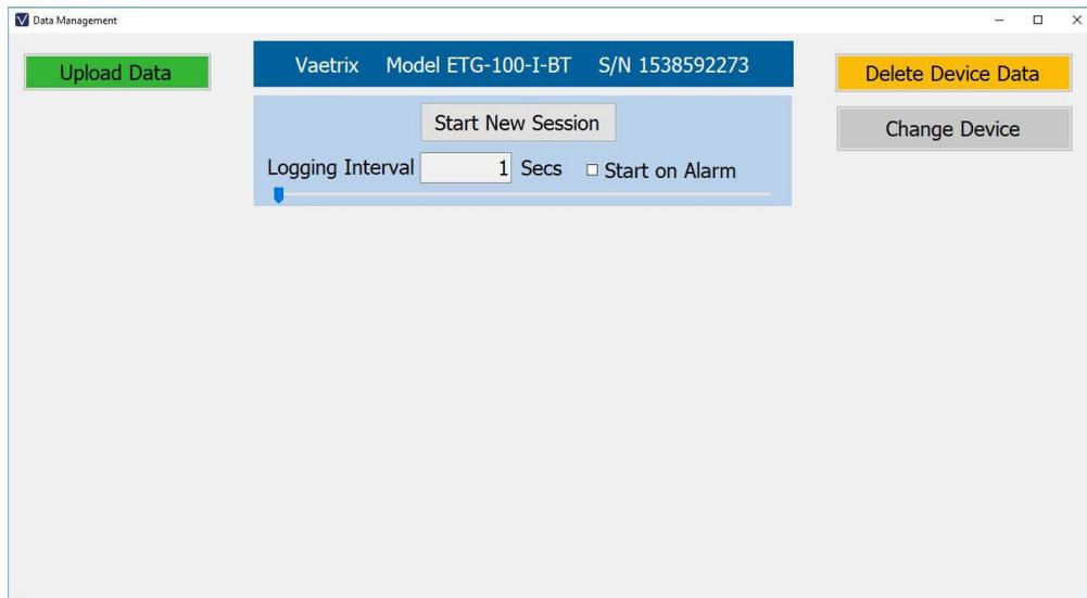
To start a new session simply use the slider bar or type in value to set the logging interval from one second to twenty-four hours and then press the Start New Session button. A session can be ended at any time by clicking Stop Session. If the High or Low Alarm values are enabled in the ETG, datalogging can be started automatically.
