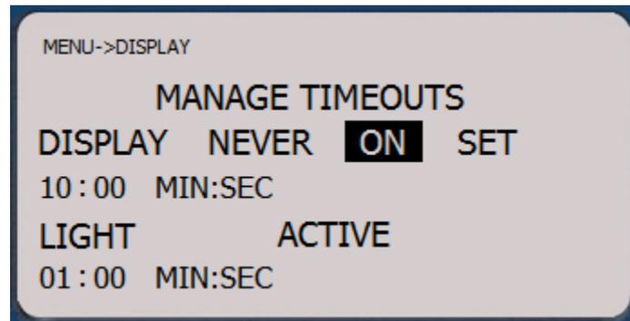
Under TIMEOUTS the DISPLAY or LIGHT can be set to turn off to conserve battery life. Intervals can be set anywhere from ten seconds to thirty minutes of inactivity.
