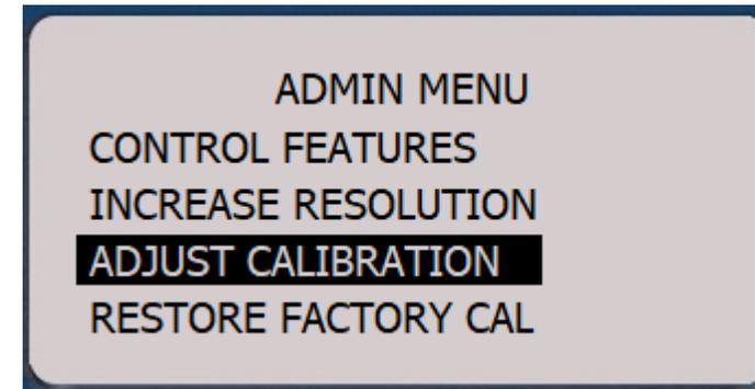
Although we suggest you return the ETG to factory for calibration, you can field calibrate the unit with trained personnel and equipment traceable to the National Institute of Standards and Technology (NIST). To begin the process select ADJUST CALIBRATION.
