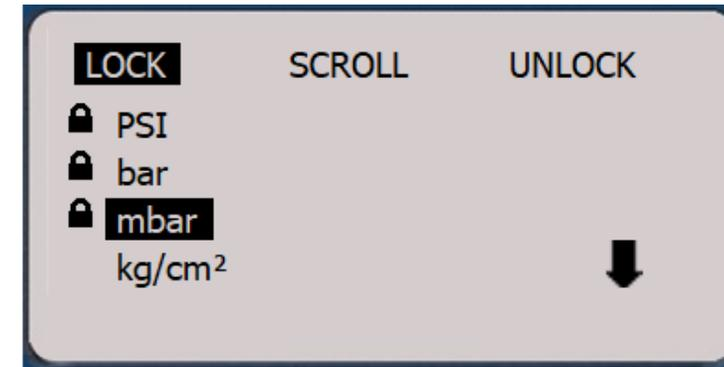
Use the right or left ARROW keys to highlight LOCK, SCROLL, or UNLOCK. Use the up or down ARROW keys to either LOCK, SCROLL, or UNLOCK the engineering units, depending on which function is highlighted.
