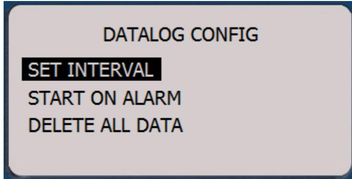
Datalogging can be setup to automatically start on an Alarm condition as well. Simply choose **START ON ALARM** and press **SELECT**. Datalogging will start based on either the High or Low alarm setting and run at the defined interval from that point forward. Clearing the alarm will not turn off Datalogging.
